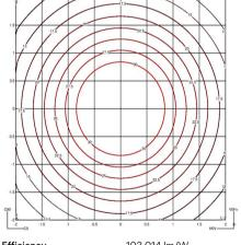
Efficiency 103.014 lm/W Coordination System CG **Total Flux** 2142.7 lm Maximum Value 103.44 cd/klm
